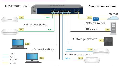
This switch is designed for indoor use only. If you want to connect to a device located outdoors, the outdoor device must be properly grounded and surge protected, and you must install an Ethernet surge protector inline between the switch and the outdoor device. Failure to do so can damage the switch.
