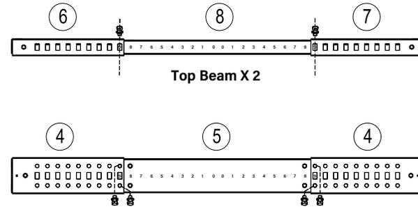
**Note:** By adjusting the beams to match the corresponding numbers marked on them, you can set the depth anywhere from 22 to 40 inches, in 1-inch increments. Please note, the actual product does not have the number 9 marked on it.
