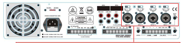
**Mute SEN –** The Mute SEN adjusts the level of override. Fully counter clockwise reduces the sensitivity where more of the bacgroung music would be heard. A high input level would be necessary to trigger the override circuit. Fully clockwise increases the sensitivity where a low input level would trigger the override circuit and the background music would be completely muted. Adjust this control to achieve your desired results.
