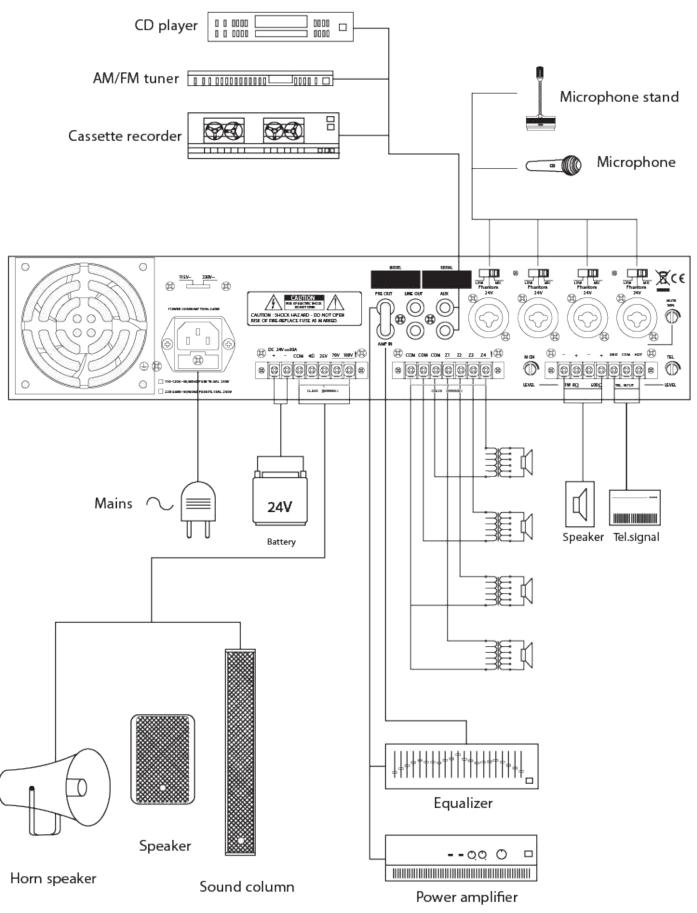
**EXPAND THE INPUTS** – It is possible to expand the inputs of the X-7240-4 using the V-RVC-PRO (remote mic/line mixer) and the X-Music (in-wall iPod Smart Phone dock). The V-RVC-PRO is capable of expanding the X-7240-4 inputs to a maximum of 12 over Cat5/6 cable. See the diagram below.
