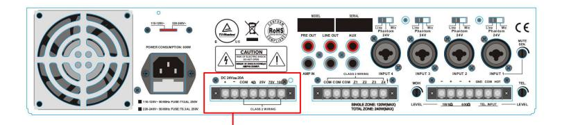
**DC 24V – 20A –** Emegency backup DC power supplies can be connected to the unit using the DC input. The DC input is polarity sensitive. Always insure the polarity of the connected power supply is consistent with the polarity of the unit.
