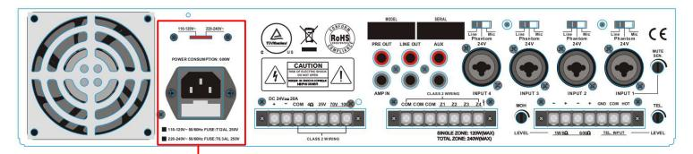
**AC Power Inlet** – Connect the supplied AC power cord in here. Only use the supplied power cord or equivilent 14awg CSA/UL approved power cord.
