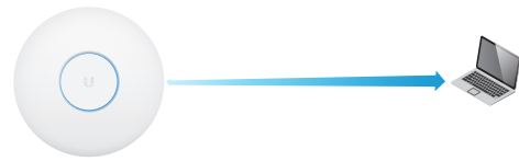
SU-MIMO: A Wave 1 AP communicates with one client at a time.
