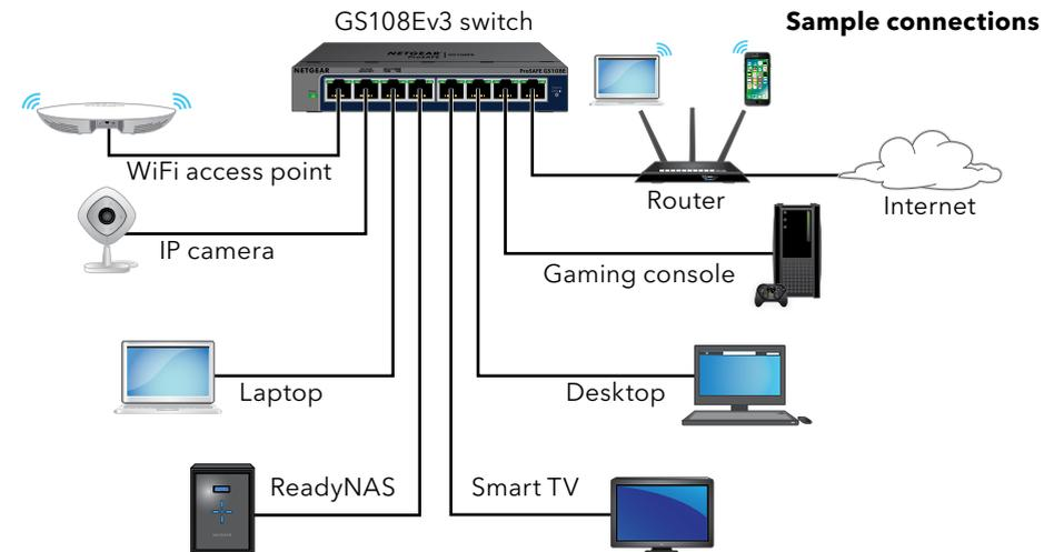
**Note:** We recommend that you use a Category 5e (Cat 5e) cable or higher-rated cable for Gigabit Ethernet connections.
