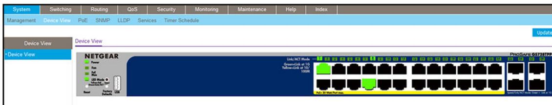
The system LEDs display on the left side on the Device View page.
