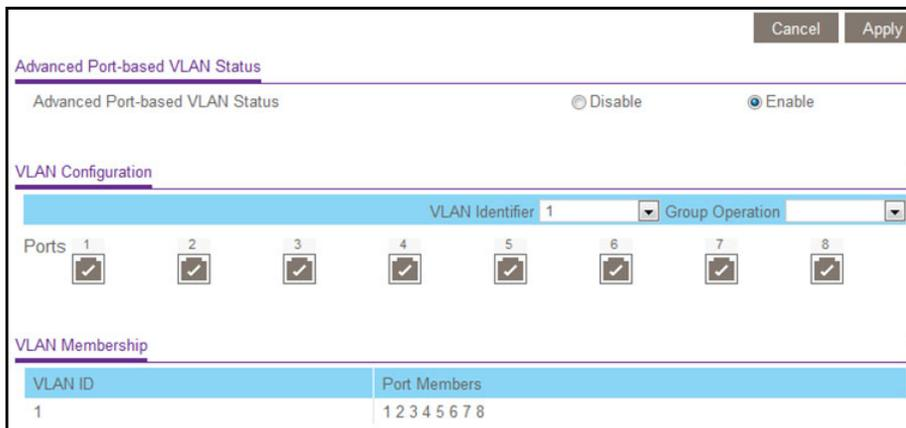
**Note:** Models GSS108E and GSS108EPP provide 8 ports. Model GSS116E provides 16 ports.
