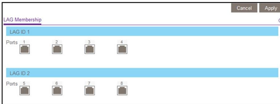
**Note:** Model GSS108EPP provide 8 ports and can support up to 4 ports per LAG. Model GSS116E provides 16 ports and can support up to 8 ports per LAG.
