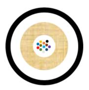
M3I-12M-P-BK fiber optic cable is constructed with twelve internal tight buffers, internal aramid yarn, and one outer plenum-rated PVC jacket in distribution format. The cable features a water-resistant jacket and is designed for indoor and outdoor applications.
