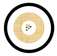
*M3I-6M-P-BK* fiber optic cable is constructed with six internal tight buffers, internal aramid yarn, and one outer plenum-rated PVC jacket in distribution format. The cable features a water-resistant jacket and is designed for indoor and outdoor applications.
