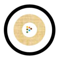
*S2I-6M-P-BK* fiber optic cable is constructed with six internal tight buffers, internal aramid yarn, and one outer plenum-rated PVC jacket in distribution format. The fiber cable features a water-resistant jacket and is designed for indoor and outdoor applications.
