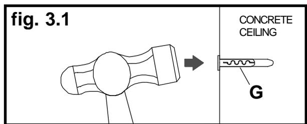
Drill holes and insert anchors (G).
