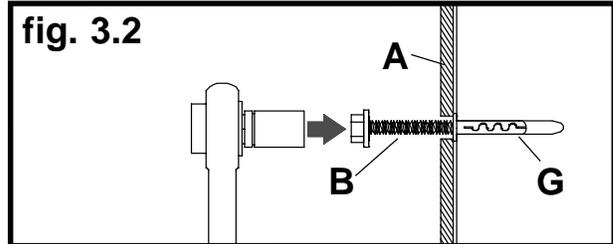
Place ceiling plate (A) over anchors (G) and secure with screws (B).
