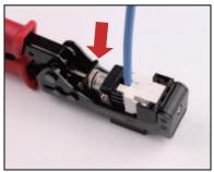
The termination/cutting depth may be varied by rotating the adjustment knobs.
