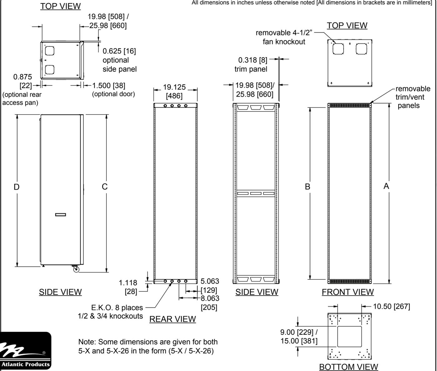
Note: Some dimensions are given for both 5-X and 5-X-26 in the form (5-X / 5-X-26)
